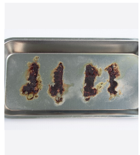
Fig. 7. ProEZ Gel™ No Bacillus Bovine Protein Soil Efficacy Test @ 72 hrs, Post-Rinse and Dry
