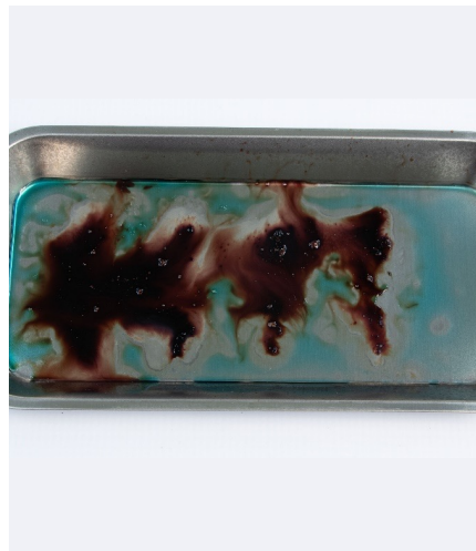
Fig. 12. Prepzyme® Forever Wet Bovine Protein Soil Efficacy Test @ 24 hrs
