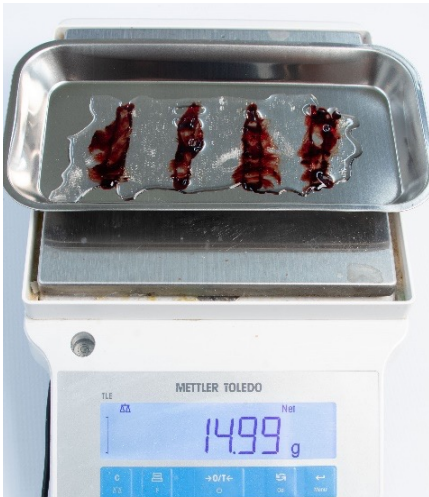
Fig. 8. PRE-Klenz® Bovine Protein Soil Efficacy Test @ 0 hrs
