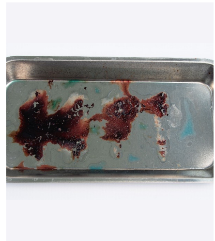
Fig. 13. Prepzyme® Forever Wet Bovine Protein Soil Efficacy Test @ 72 hrs, Post-Rinse and Dry
