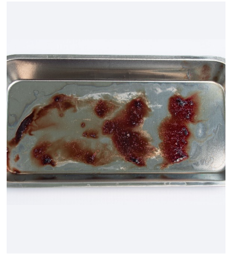
Fig. 10. PRE-Klenz® Bovine Protein Soil Efficacy Test @ 72 hrs, Post-Rinse and Dry
