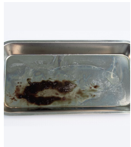
Fig. 16. OptiPro® Bovine Protein Soil Efficacy Test @ 72 hrs, Post-Rinse and Dry
