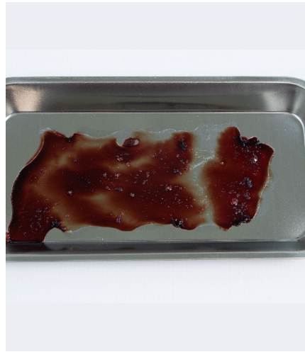
Fig. 9. PRE-Klenz® Bovine Protein Soil Efficacy Test @ 24 hrs
