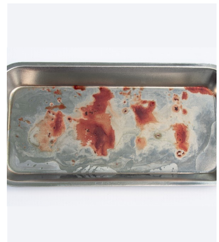
Fig. 4. ProEZ Gel™ Bovine Protein Soil Efficacy Test @ 72 hrs, Post-Rinse and Dry
